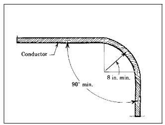
**Figure 7.** Ground Cable. The ground cable should take as direct and straight a line as possible from the mast top to the water ground. No bends exceeding 90 degrees with an 8 inch minimum radius should be used.
