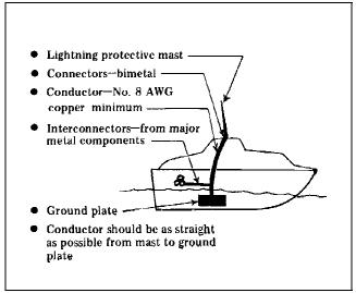
Figure 5. Components of a Lightning Protection System.
